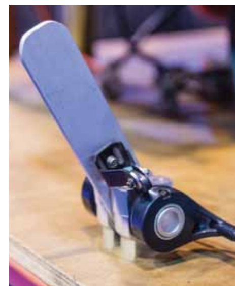
Above: Front flexible coupling clearly seen below the propeller shaft Left: Throttle assembly, using a pair of mobility scooter speed controllers Right: An early run, before we discovered the missing boost pressure
