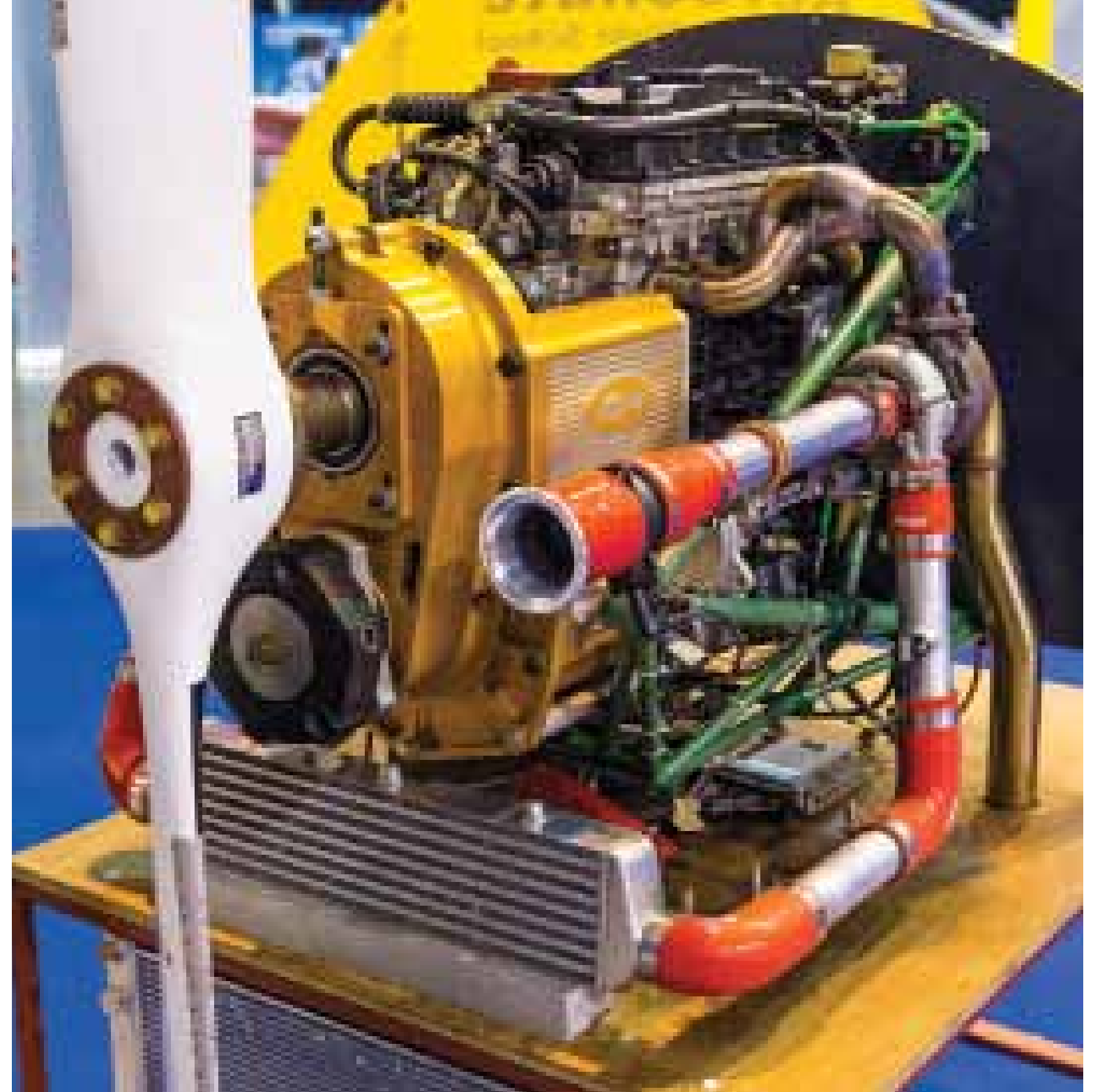
Above: Front flexible coupling clearly seen below the propeller shaft Left: Throttle assembly, using a pair of mobility scooter speed controllers Right: An early run, before we discovered the missing boost pressure
